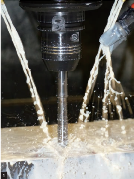
1. The OSG Phoenix PFB indexable ball end mill nearly tripled cycle time and doubled tool life while significantly improved surface quality in Stickel's metal mold application.
