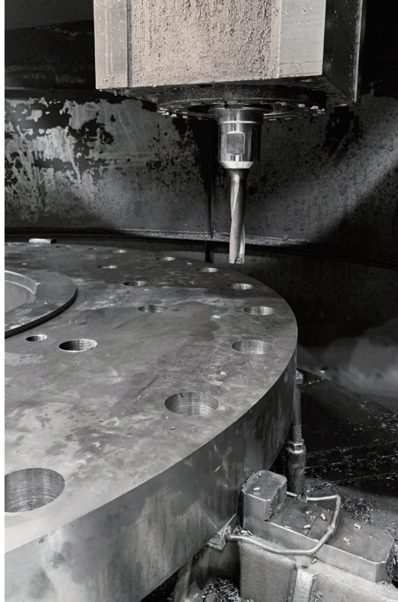
The OSG Phoenix P5D indexable drill is used to drill holes in GIW's production of slurry pumps made of cast steel and ductile iron.
