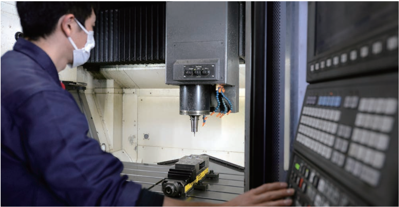
Takaki Kanagata machine operator Yuichi Ishikawa prepares for the milling of OSG's custom Tap-kun plastic model mold made of STAVAX.
