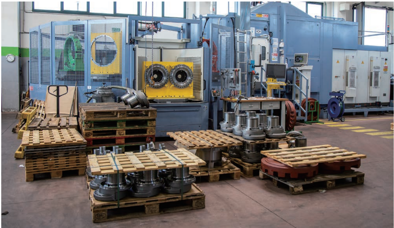
MPC's MCM Tank horizontal machining center with HSK-A100 holder that is used for processing planetary bearing hubs for gearmotors.
