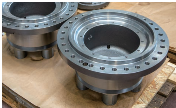
Components for gearboxes made of GS-600 cast iron. Each part requires the threading of 30 holes in the size of M24 x 3, tolerance 6HX and at an axial depth of cut of 40 mm (through hole).
