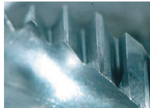
Cutting Edge after Tapping 1,000 Holes
