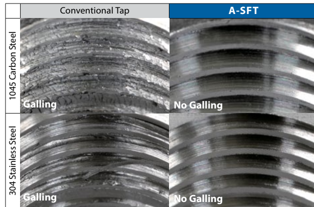
Visual Reference of Internal Threads. (Results may vary based on machining conditions.)
